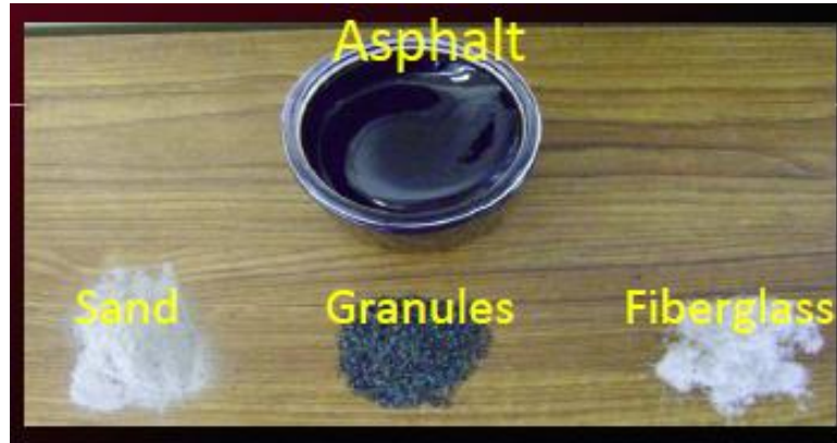
Figure 2-1. Components of Asphalt Shingles (Grzybowski et al. 2010)
